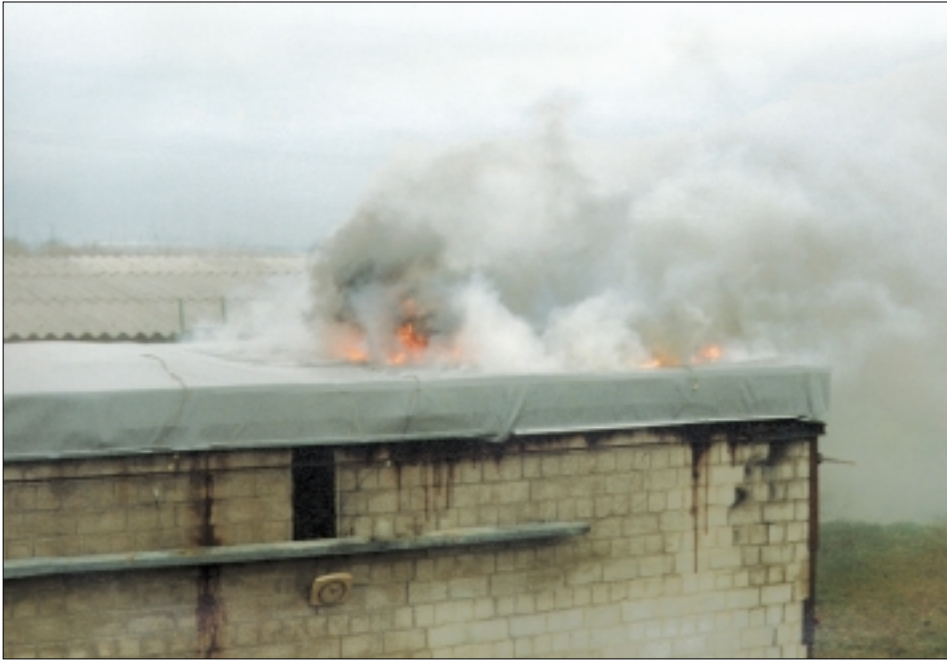
Figure 4: Roof during fire test - Pentane blown foam
