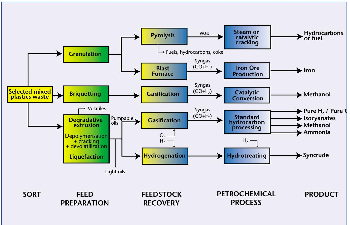
Possible chemical products obtained through feedstock recycling
