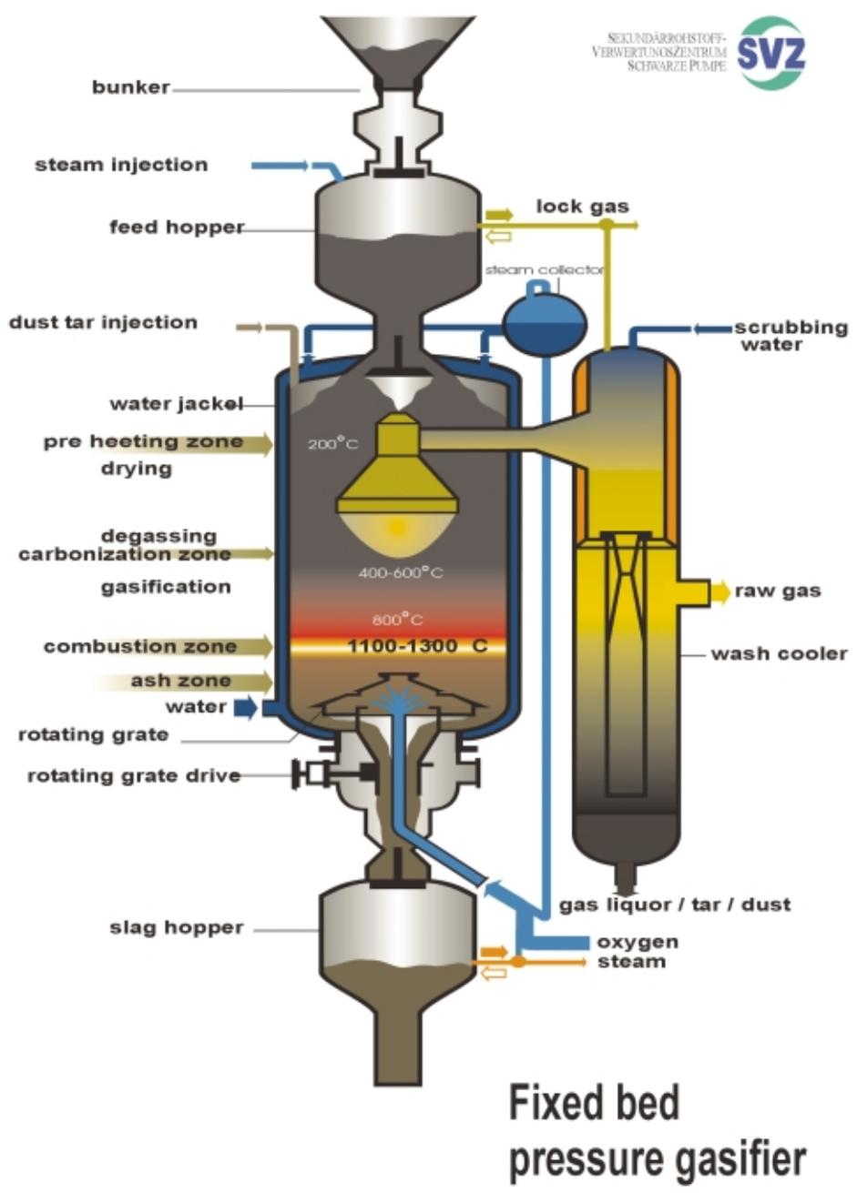
*Schematic of the SVZ fixed bed pressure gasifier*
